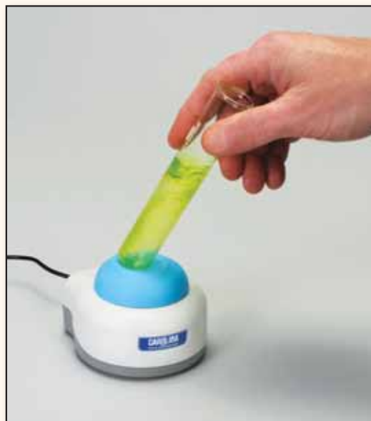
A special machine called a vortex mixer is used to shake the sample.
