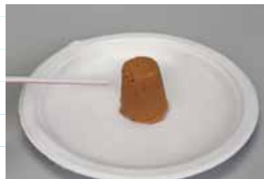
Figure 2.2 A sand tower with a straw for the wind test
